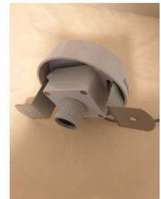
Mount the sensor so it is perpendicular to the level being measured. It is possible to narrow the beam by placing a 32mm conduit fitting over the sensor head, in this case the perpendicular requirement becomes much more important.
